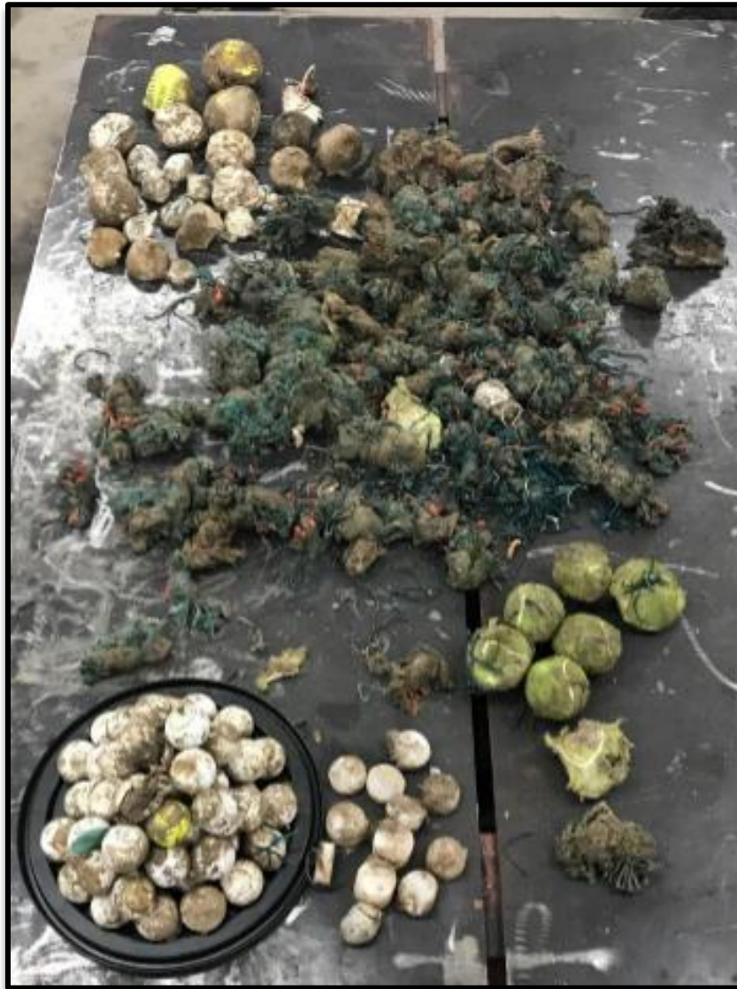
Figure 14: Recovered Junk Shot from a well Blowout
