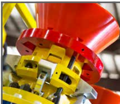
PRIMARY CAM LOCKS SECURE THE CONNECTION AND ARE LOCKED OUT WITH A SECONDARY RING.
