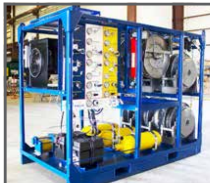
RIGLOCK™ SYSTEMS ARE CONTROLLED WITH A CUSTOM-DESIGNED HYDRAULIC CONTROL UNIT.
